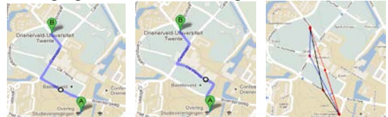
Fig. 1. Figures in left and middle show two possible paths between A and B. Figure in right shows three different trajectories between point A and B resulted by interpolation. Black and red trajectories, each follow one of these paths and the blue trajectory is not even classifiable by human eye.
